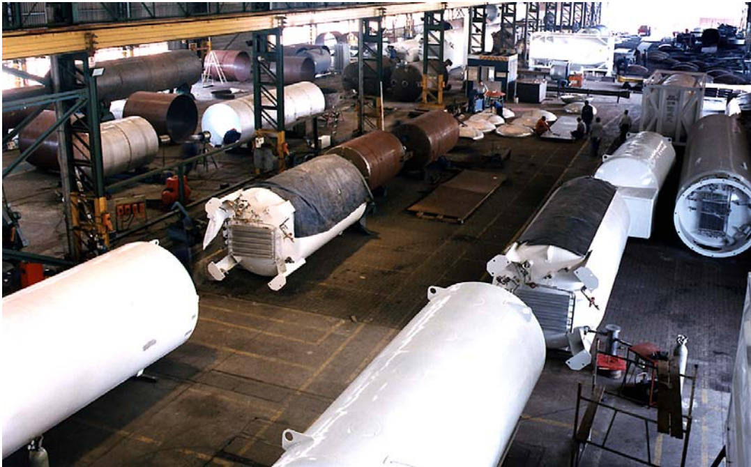
Manufacturing vertical, vacuum insulated storage tanks.
